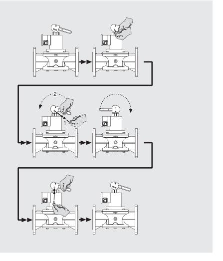
Manually operated safety shut-off valve HSAV/5
