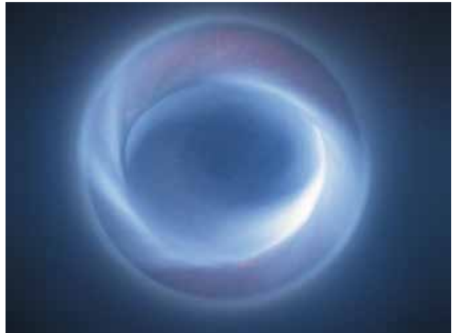
Lean gas flame with a LHV of 3 MJ/m 3 : The combustion of a SAACKE lean gas burner is so clean and stable because of the intensive mixing of fuel and air with low pressure loss.
