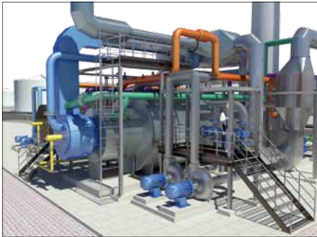
Thermal oil heater plant with lean gas burner in Rotterdam
